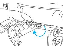
If the tether strap is clipped incorrectly (as shown) the child safety seat may not be retained properly in the event of a collision.
